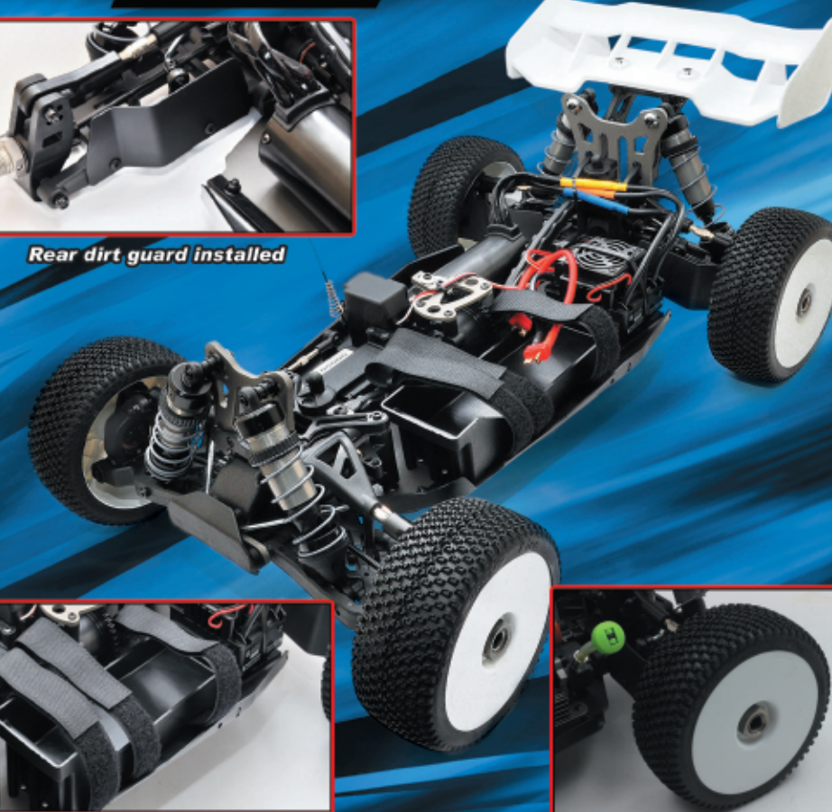
L-pin treads w/ instant grip and acceleration
