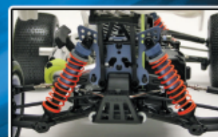
Front / rear aluminum shocks
