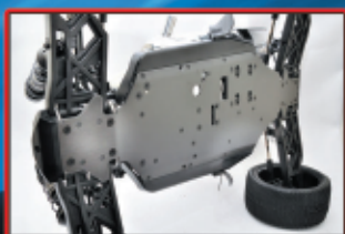
Aluminum chassis with adjustable down travel
