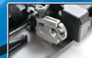
CNC aluminum motor mount and sealed receiver box
