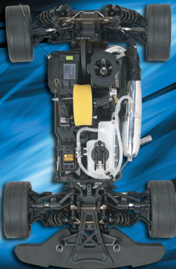
High impact front foam bumper
