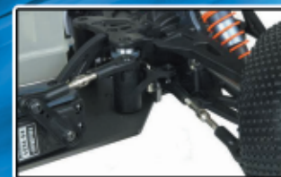
Aluminum adjustable turnbuckles throughout the car
