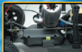
Sealed waterproof battery/receiver box
