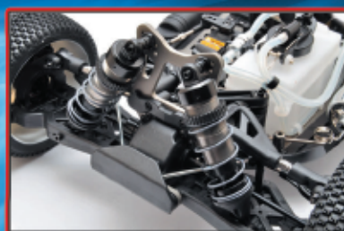
17mm big bore aluminum adjustable shocks
