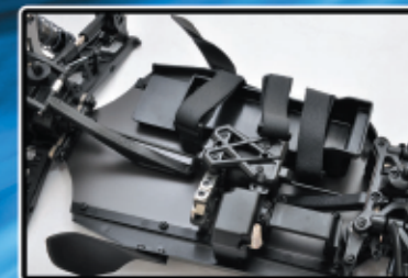
One piece molded battery case with ESC pedestal and battery straps
