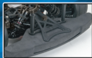
High impact front foam bumper
