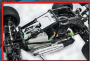
Aluminum roll cage provides protection against collisions
