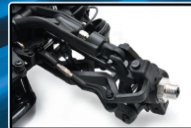
New front C-Hub suspension design with constant velocity CVA shafts
