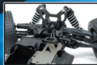
Front / Rear CNC aluminum shock tower and radio tray
