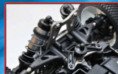
17mm big bore aluminum adjustable shocks
