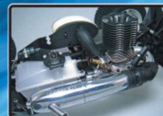
Aluminum racing manifold and exhaust installed
