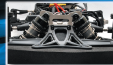
Cnc aluminum front shock tower and high impact foam bumper
