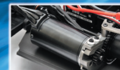
2000kv motor and CNC aluminum motor mount
