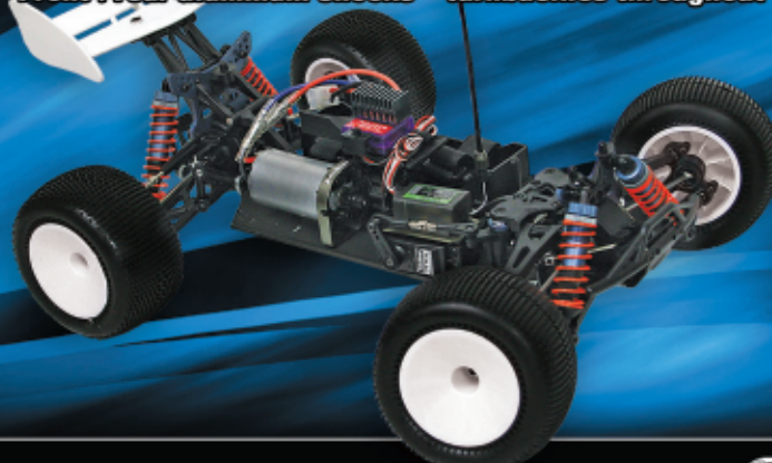
Front / rear aluminum shocks
