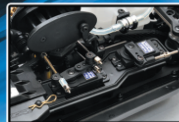
18 kg / 252 oz digital metal gear waterproof servos (USA) installed on one piece radio tray
