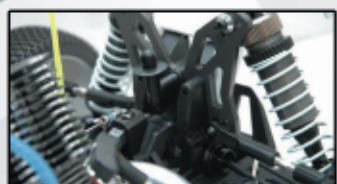
Big Bore 20mm aluminum adjustable shocks bolted to CNC aluminum shock towers
