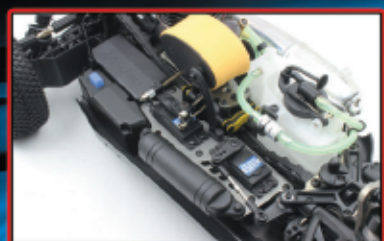
Adjustable battery location
