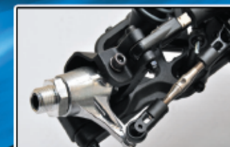
Aluminum steering knuckle w/ front CVS shafts
