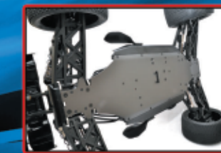
One piece aluminum chassis with adjustable down travel.
