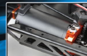
Full aluminum roll cage protecting brushless motor
