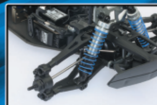
Front / Rear CVA universal swing shafts
