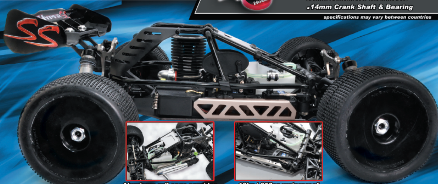
Aluminum roll cage provides protection against collisions
