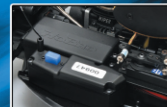
Sealed waterproof receiver / battery box
