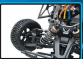
Aluminum adjustable big bore shocks
