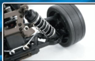
Adjustable big bore aluminum shock system
