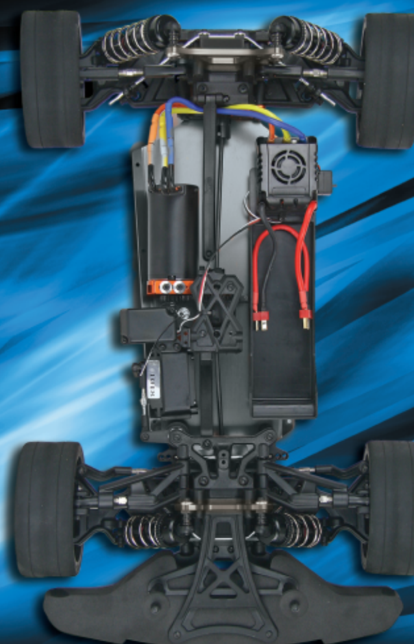
CNC aluminum motor mount and sealed receiver box
