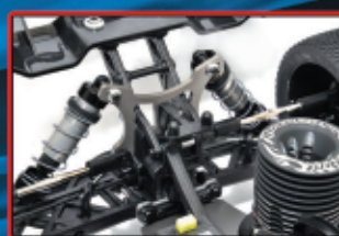
Front | Rear aluminum shock tower w/ chassis braces
