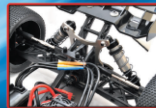
Front | Rear Aluminum Shock Tower w/ Chassis braces
