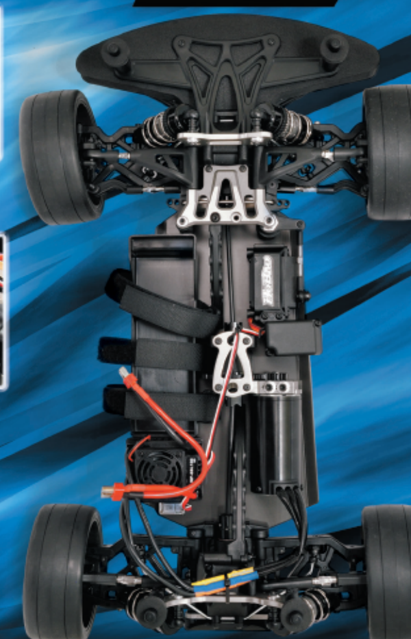
Cnc aluminum front shock tower and high impact foam bumper
