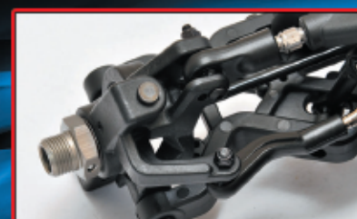
Front C-Hub suspension with CVA shafts
