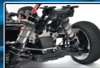
Front / rear anti-roll bar
