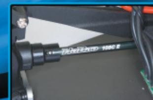
Universal Center shafts w/ laser engraving
