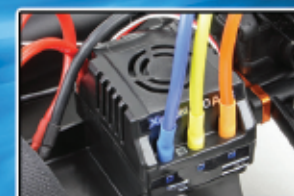
HobbyWing Waterproof brushless Speed Control
