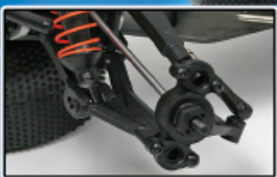
Pivot ball suspension w/ front CVD
