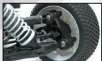
World champion proven pivot ball suspension (PBS)
