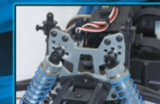
Aluminum Front/Rear Shock tower with adjustable geometry
