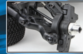
Front C-Hub suspension with CVA shafts
