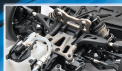
Cnc aluminum front top plate and front shock tower
