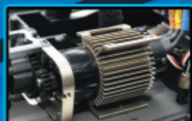
Brushless 2200KV motor w/ aluminum cooling fins
