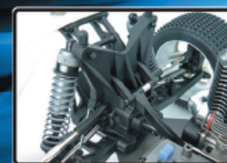
Light weight molded shock tower and chassis braces
