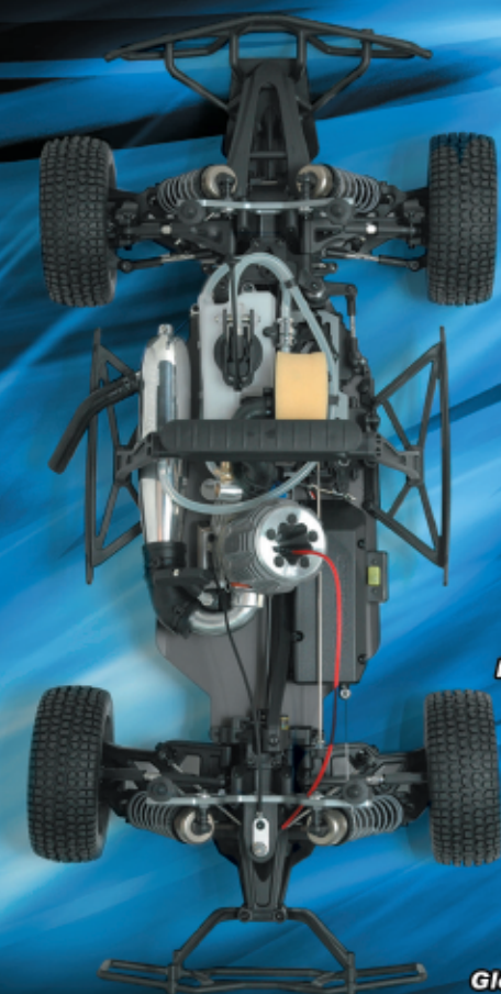
Sealed waterproof battery/receiver box
