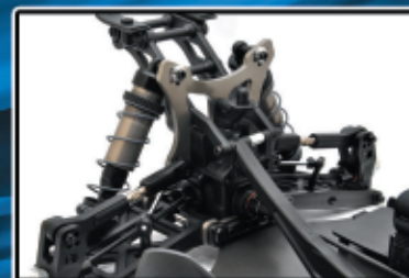
Front / Rear chassis braces
