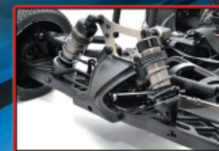
17mm big bore aluminum adjustable shocks
