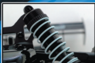
Big bore 20mm aluminum adjustable shocks
