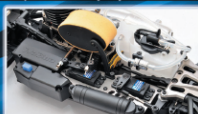
Sealed receiver box with adjustable battery position
