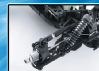
Aluminum spindle with front CVA shafts
