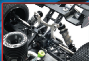
Reinforced suspension arms and turnbuckles
