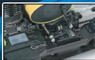
One piece upper deck with sealed receiver and battery box
