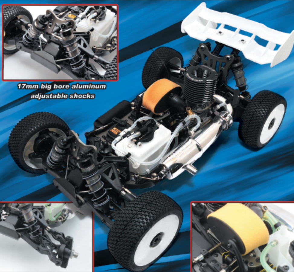
Front C-Hub suspension with CVA shafts
