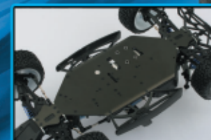
Hard anodized one piece aluminum chassis
