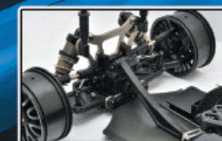
Front and rear aluminum shock towers and composite chassis braces
