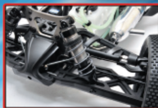
17mm big bore aluminum adjustable shocks
