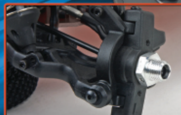
Front C-Hub suspension with CVA shafts
