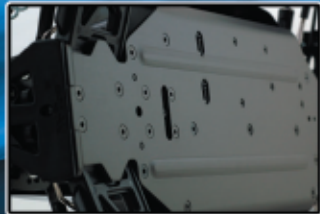
Reinforced CNC one piece chassis with adjustable down travels
