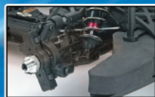
King Pin front steering system
