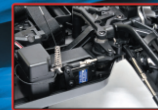
18kg | 252oz waterproof metal gear digital servo
